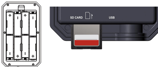
Figure 5: Installation of batteries and SD card
