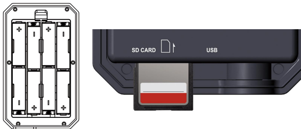
Figure 5: Installation of batteries and SD card
